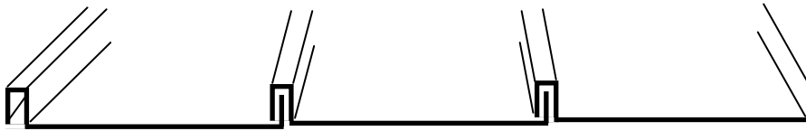
Roof Panels Overlap Each Other
